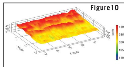
The powerful PC software allows an overlapping of the moisture and permeability profiles taken by both instruments, allowing an immediate troubleshooting of the felt bands and barring, using the instrument scans taken during the normal routine service, at no extra time
