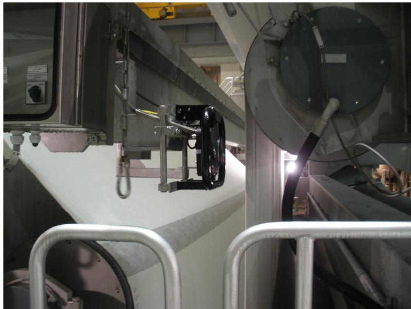
**Figure 3.** The traversing and fully programmable felt scanner
