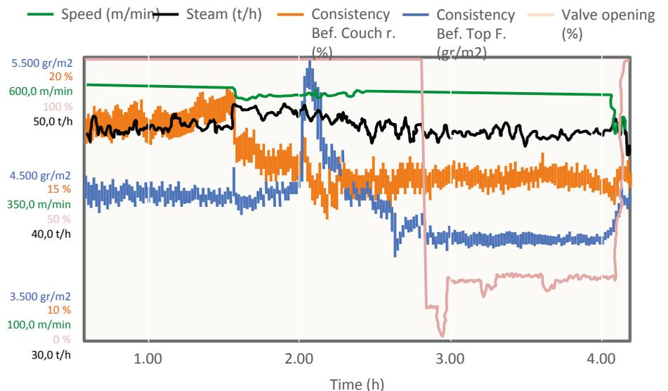
Figure 14. Water content (blue) without control mode (left and center right) vs. in control mode (lower right). Variability is greatly reduced.
