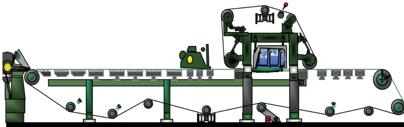
Figure 13. The dewatering units
