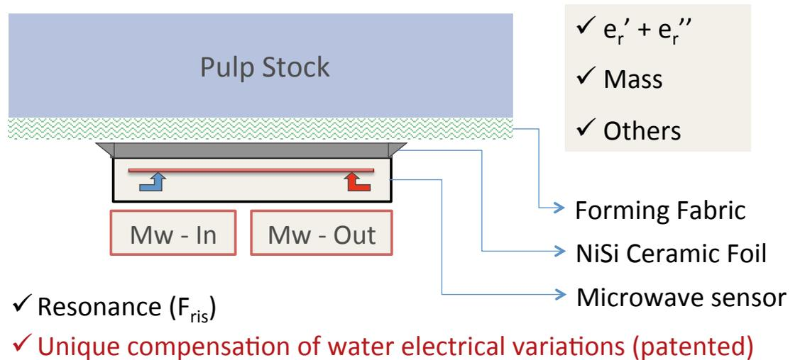
Figure 1. New planar sensor operates without a resonance chamber
