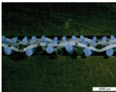
**Figure 3.** shows the same ESB structure utilising same sized MD/CMD yarns, but with a longer float weave pattern on sheet side to retard drainage rate.
