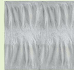
Fig. 5 (left) shows the paper surface; the phenomenon was described as paper mass variation, moisture and caliper streaks. These streaks were fluctuations of the basis weight in machine direction, completely parallel, always the same distance over the paper width. The darker streaks were clearly related to higher basis
