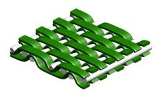
**DuraTier™** is a dryer fabric expressly designed for unirun groups: double layer, symmetrical design, with flat PET monofilaments MD and round PET monofilaments CMD.
