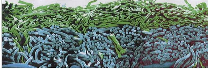
**HydroSmooth™** press fabric has been engineered for positions where sheet smoothness is essential. The special micro-needling, batt fibre orientation and possible use of **QuadraTech™** flat fibres, allows excellent levels of sheet smoothness.
