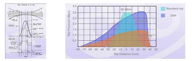
The high compressibility of **MicroPrexx<sup>™</sup>** allows a low thickness (faster water flows transfers) felt under the higher pressure in the first part of the nip for an efficient dewatering; when its elasticity recovers full thickness in the depressed end of the nip, slowing down flow transfers, thus rewetting. In addition the Interface<sup>™</sup> layer contributes to strongly break down the possible rewetting water.
